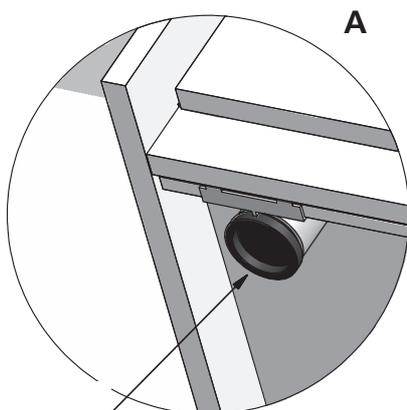
Use the height adjustment elements of the cabinet to adjust any imbalances in the floor.
