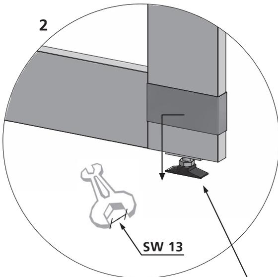
Afterwards, adjust all frames and slide the cover until it reaches the flooring.
